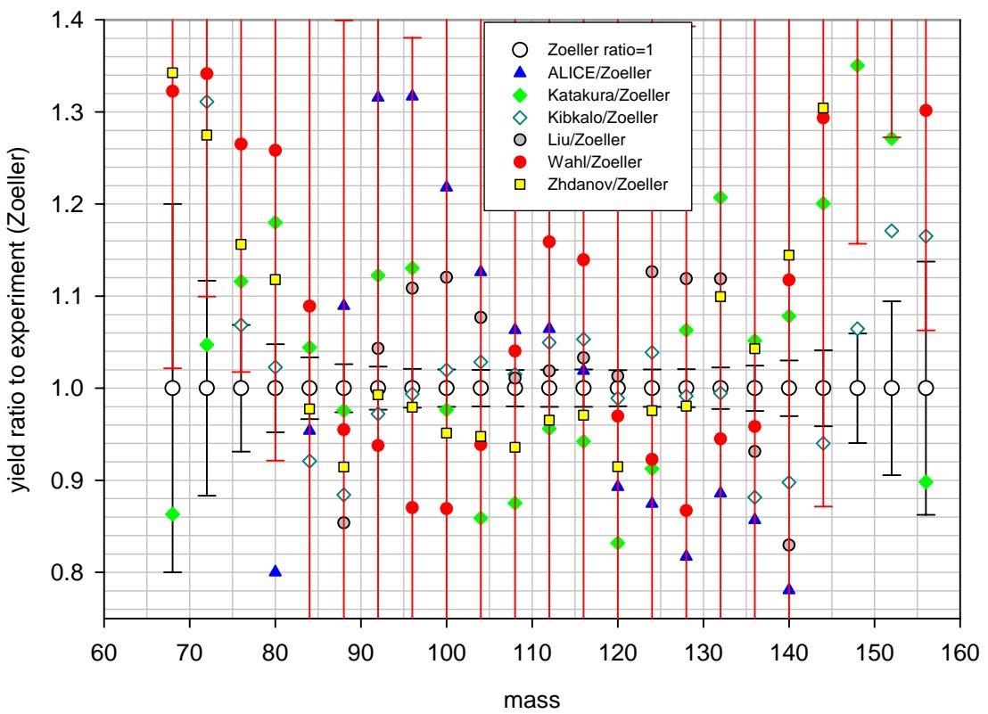
Benchmark A:  $^{238}\text{U}$  at 160 MeV, post neutron emission yield ratio to experiment (Zoeller)
